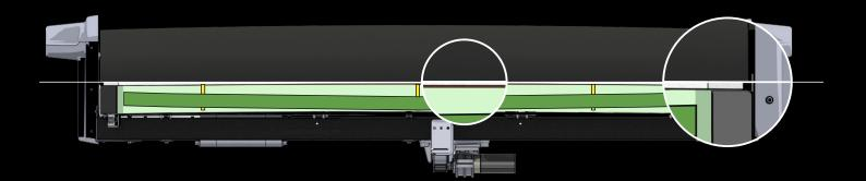
Perfectly flat when roller is lowered - this is the key to a reliable applicator. Our (patent pending) solution using two internally embedded beams gives incredible reliability and stability to the table...
